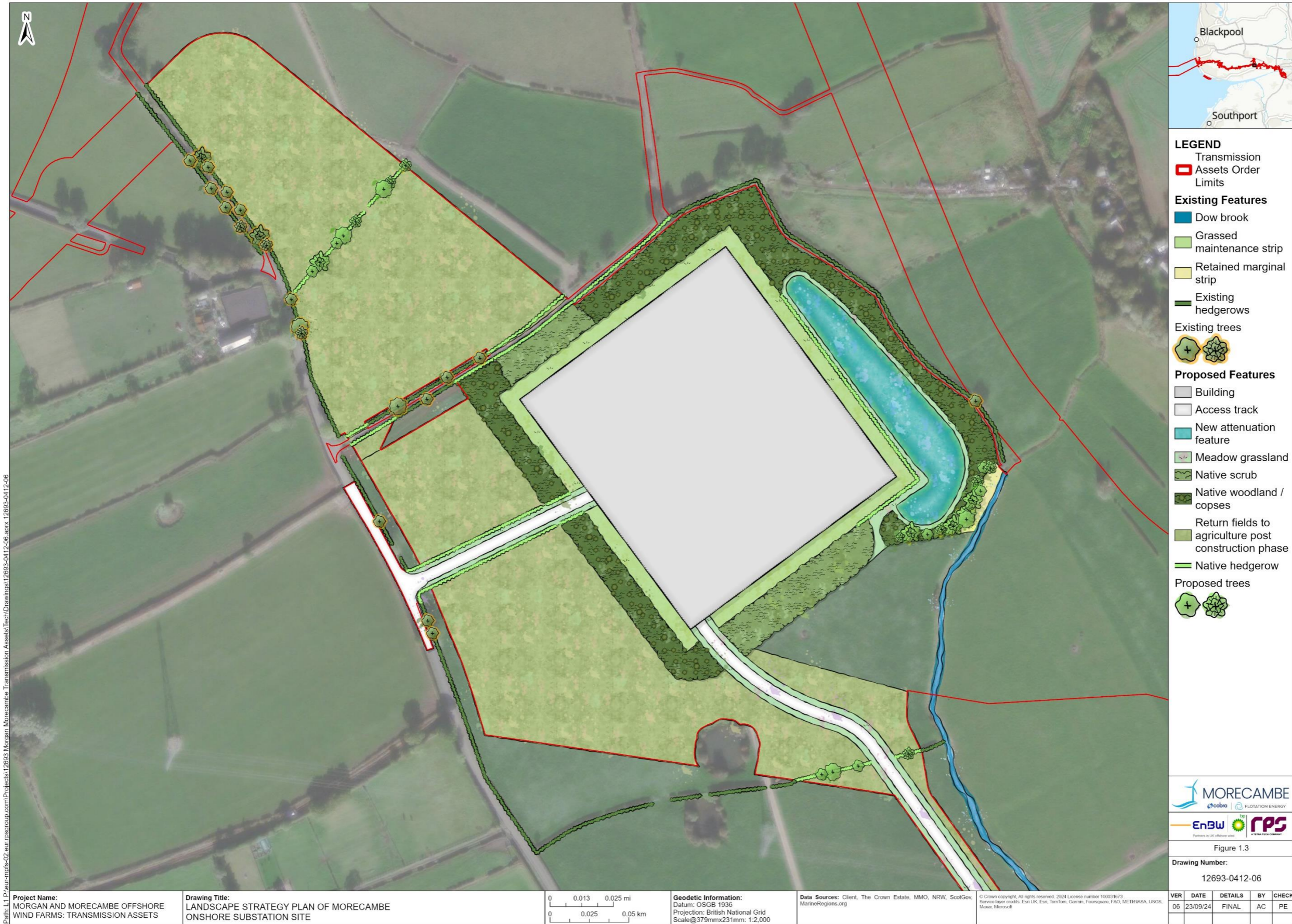
Figure 1.3: Landscape strategy plan of Morecambe onshore substation site
